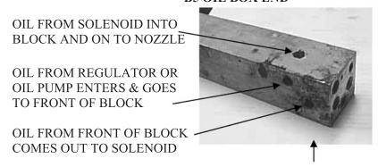
UNDER BLOCK IS TAPPED PORT FOR AIR FROM REGULATOR TO GET INTO BLOCK
