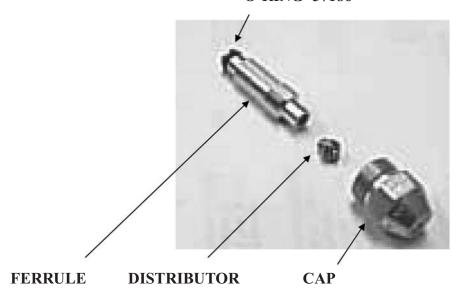
For a more thorough service the following burner components can be cleaned as a preventative yearly maintenance.
