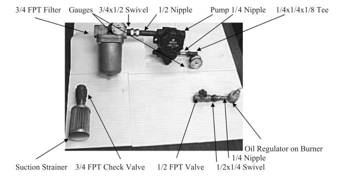
**Suction Line:** Field provides piping from Check Valve to Filter. Secure piping to keep the Suction Strainer 6 inches off the bottom of the tank in order to avoid water and antifreeze pickup from the bottom of the oil tank. Plan ahead for routine service of components. Use minimal number of fitting to reduce chances of suction leaks. Note: Some J Pumps have dual suction ports. It is only necessary to pipe to one of these 1/2 inch ports.
